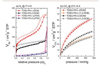
Fig. 5 N<sub>2</sub> (77.4 K) (a) and CO<sub>2</sub> (273 K) (b) adsorption/desorption isotherms (adsorption with filled spheres, desorption with hollow spheres) of various TOSU-PA-c/TOSU-PA-d materials synthesized under different conditions.
