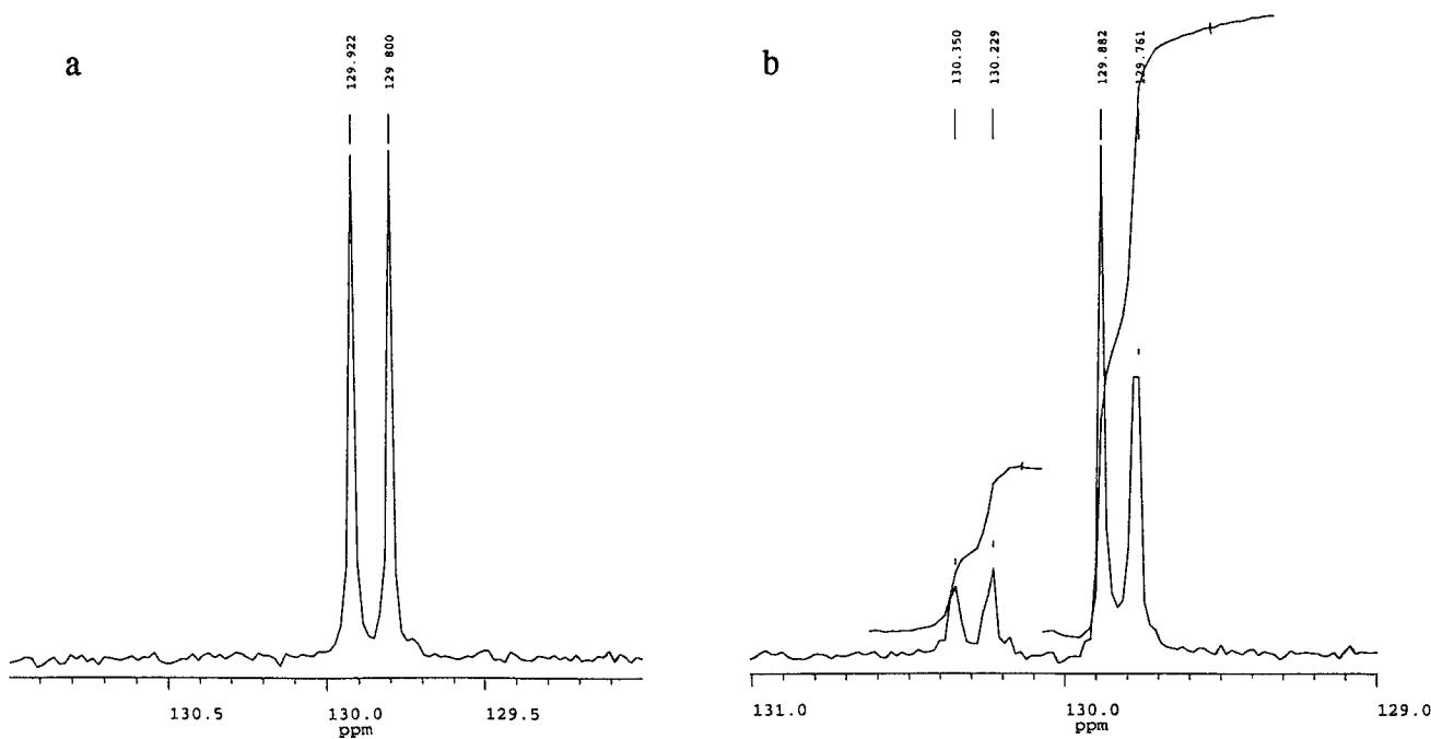
Olefinic region in the  $^{13}\text{C}$  NMR spectrum of compound **16** prepared (a) by the boron-reaction manifold according to Scheme 2, (b) by Lindlar hydrogenation according to Scheme 6.
