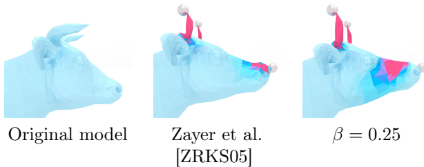
Figure 4: Cow . The handle on face is fixed, and the horns are rotated upwards. Regularization helps preserve the volume near the base of the horns.
