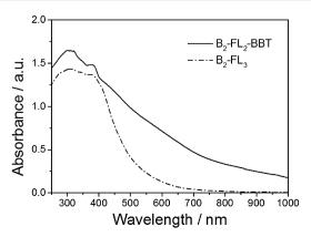
Fig. 2 UV/Vis DRS spectra of B<sub>2</sub>-FL<sub>2</sub>-BBT and B<sub>2</sub>-FL<sub>3</sub>.
