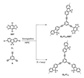
Scheme 1 Synthetic route and idealized structure of B<sub>2</sub>-FL<sub>2</sub>-BBT and B<sub>2</sub>-FL<sub>3</sub>. Reaction conditions: (i) Pd(PPh<sub>3</sub>)<sub>4</sub>, Cul, K<sub>2</sub>CO<sub>3</sub>, span 80, toluene-H2O (v/v: 1/9), 80 °C, overnight.
