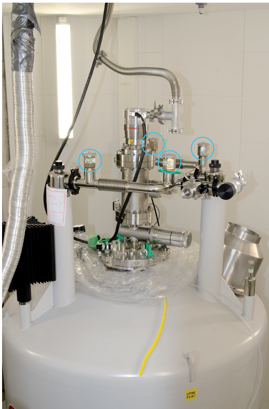
Figure A.3: PENTATRAP magnet with safety valves indicated in blue. These valves open at an overpressure of about 200 mbar.
