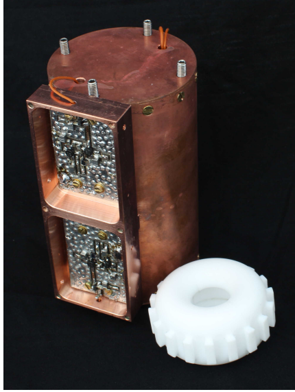
Figure 3.21.: Two assembled axial detectors (with amplifier box lid removed) in a double-resonator housing, as well as a toroidal PTFE coil body are shown. The coils are made from PTFE-insulated 75 \mu\text{m} thick NbTi-wire, wound on the coil body. The torus is wrapped in PTFE-tape for mechanical stability of the coil. For further details see text.
