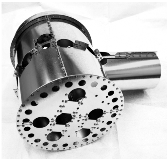
Figure 3.6: Photograph of the preassembled mu-metal hull before it is mounted around the main vacuum tank. It consists of seven large and several small individual pieces.
