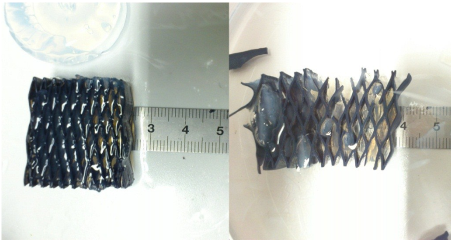
Figure 39. Hydro-actuated hydrogel-filled-honeycomb structures. Swelling of superporous poly-acryl-co-acrylamide hydrogels inside the diamond shape cells of a 3D printed honeycomb structure result in ~65% expansion of the cells along the shorter transverse cross-section direction. The poor control over constraining the hydrogel inside the honeycomb cells, made it difficult to achieve a quantitative analysis of the system.
