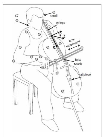
FIGURE 1 | Illustration of setup, instrument, and task. Marker positions are indicated as gray circles. The cello-centered coordinate system is indicated (note that the actual origin was defined to be at the scroll marker). Reproduced with permission from Verrel et al. (2013).
