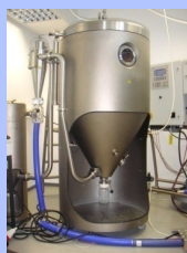
Spray drying in technical scale for rapid and continuous solidification and drying.
