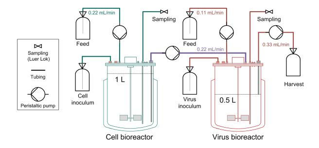
Figure 4.40.: Reactor setup for continuous influenza A virus infection. The setup comprises two stirred tank reactors in which AGE1.CR suspension cells were cultivated in continuous mode. Both reactors were connected via the purple tubing such that cells were constantly fed into the virus reactor where infection took place. Green components belong to the cell reactor and red components to the virus reactor. Figure taken from Frensing and Heldt *et al.* [148].
