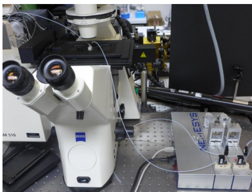
Figure 5.1: The image shows the flow cell being attached simultaneously to a syringe pump and to the sample holder of the confocal microscope.
