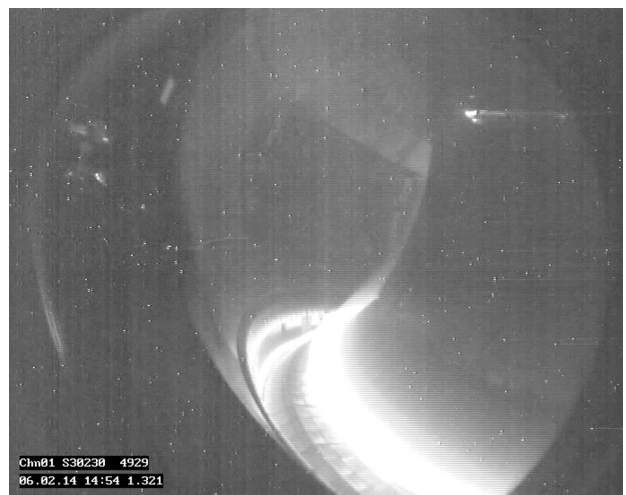
Figure 11. Video snapshot from AUG experiment #30230. In the upper right corner an arc can be seen on the HS. This was ignited by an ECRH beam shine through. Under normal conditions this area is dark. Most of the light comes from the divertor region at the bottom of the machine.
