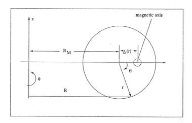
Figure 16: Tokamak with shifted circular surfaces
