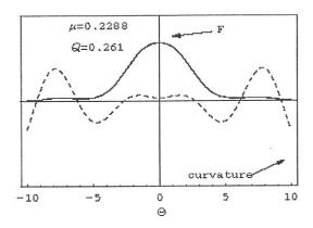
Figure 9: Eigenfunction for S = 1.0, m = 235 and n = 0.
