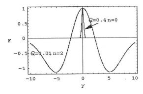
Figure 1: Dispersion relation in cylin. geometry.
