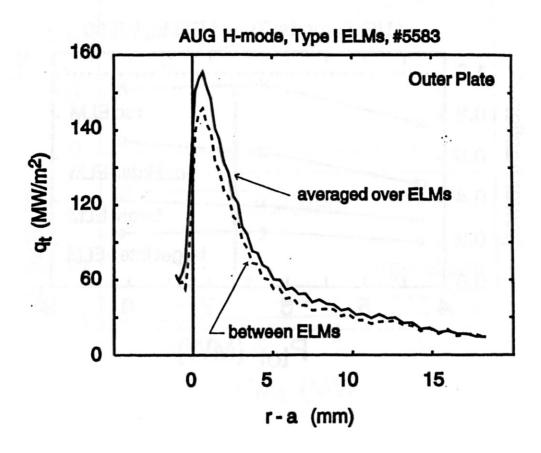
12. Parallel power density from IR thermography at the outer plate between ELMs and time-averaged over ELMs (shot 5583).
