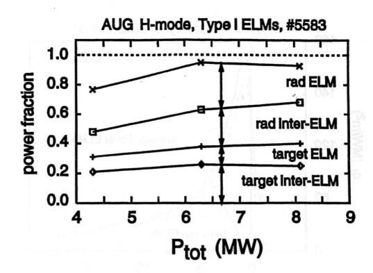
11. Power balance in a discharge (5583) with varying heating power and Type I ELMs. The fractions of radiated power, powers deposited on the plates, during or between (inter) ELMs.
