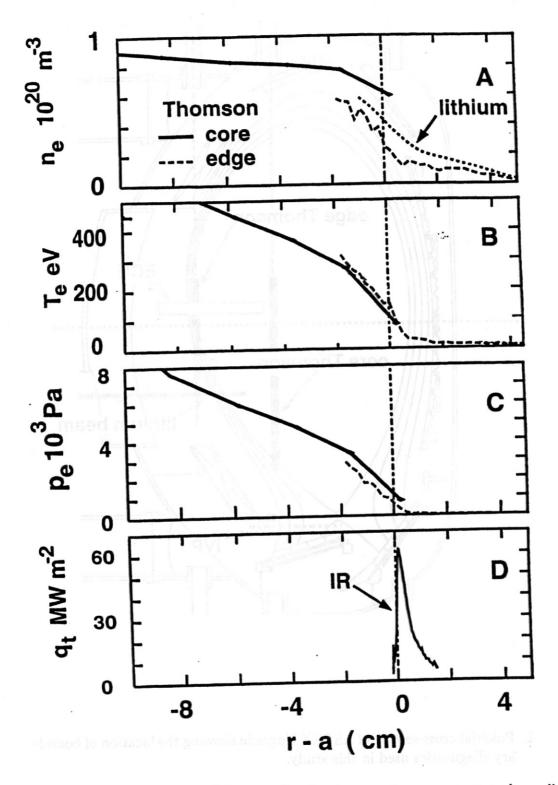
2. Typical profiles of electron density, temperature, pressure and parallel power from two identical H-mode discharges (shots 7985, 7994) with  $I_p = 1.0MA, B_t = 2.5T, \, \overline{n}_e = 8 \times 10^{19} m^{-3} \, \text{and} \, P_{NBI} = 5.0MW$ . All measurements are mapped to the outside midplane.
