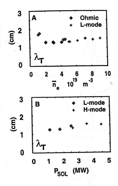
6. The temperature e-folding width  $\lambda_T$  (mapped to the mid-plane) from ECE measurements under a range of conditions.
