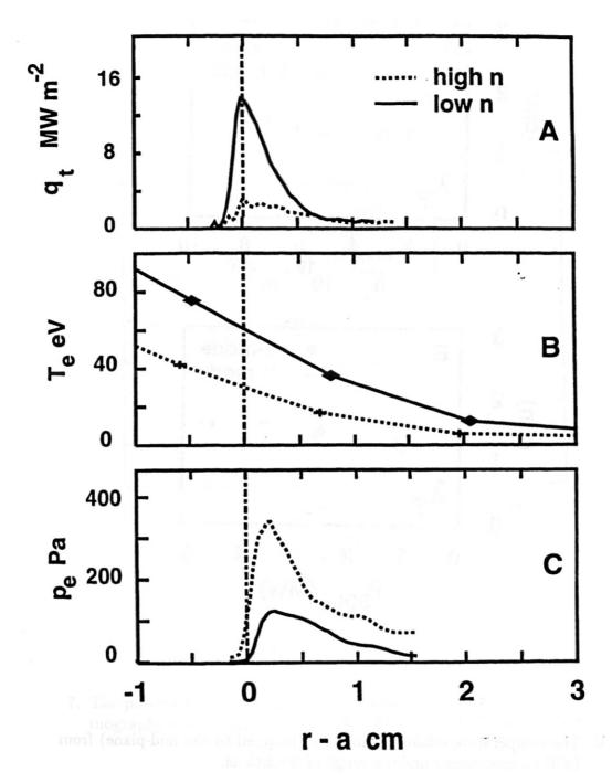
5. Comparison of (a) plate profiles of deposited power with (b) upstream measurements of  $T_e$  from ECE for low and high density Ohmic discharges (5944, 5946). Also shown in (c) are electron pressure profiles obtained with a moving Langmuir probe located mid-way between the plate and the X-point. (a) and (c) correspond to the outer divertor.
