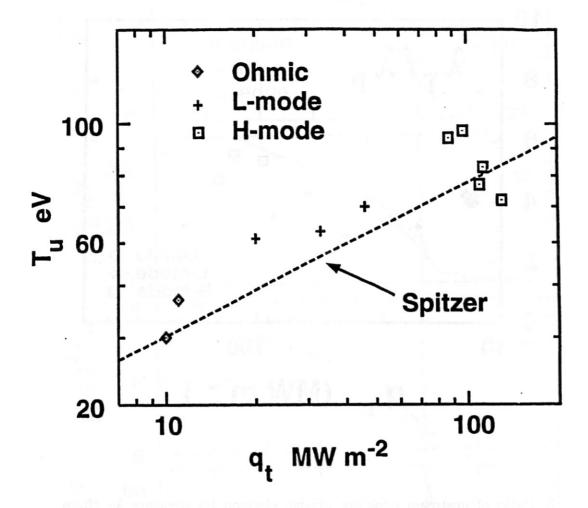
4. Upstream electron temperature  $T_u$  from Thomson scattering as a function of parallel power density  $q_t$  from IR thermography (outer plate) in low radiation discharges (7808, 7810). Also shown is an absolute comparison based on Spitzer-Härm conductivity.
