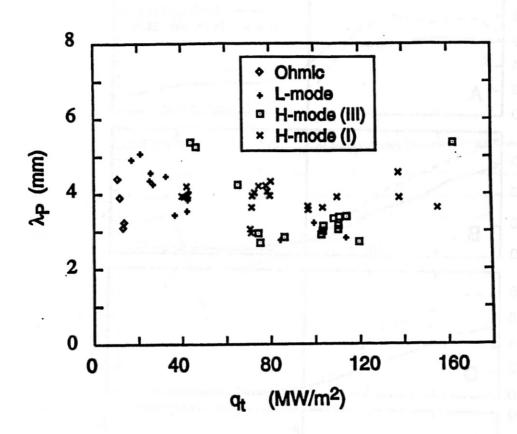
7. The power e-folding width  $\lambda_P$  (mapped to the mid-plane) from IR thermography measurements at the outer plate in low radiation discharges.
