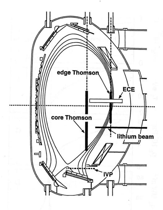
1. Poloidal cross-section of ASDEX Upgrade showing the location of boundary diagnostics used in this study.
