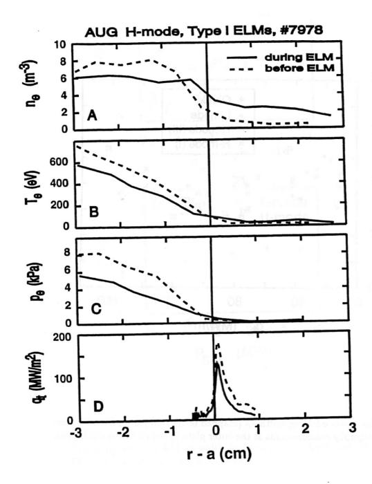
8. ELM-resolved SOL profiles of electron density, temperature and pressure from Thomson scattering in a low radiation H-mode with Type I ELMs (shot 7978, t = 2.5s to t = 3.5s). Also shown in (d) are the corresponding parallel power density profiles from IR thermography (outer plate).
