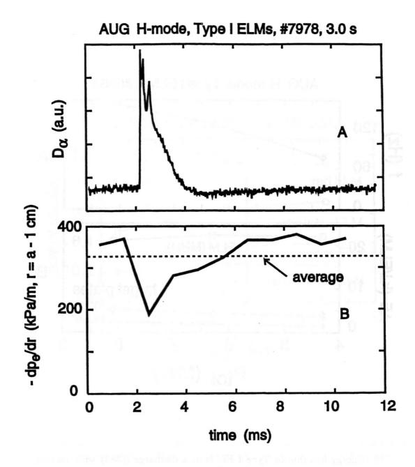
9. The divertor  $H_{\alpha}$  time behaviour and the corresponding electron pressure gradient derived from Thomson scattering at r = a - 1cm for the same discharge as depicted in Fig. 8.
