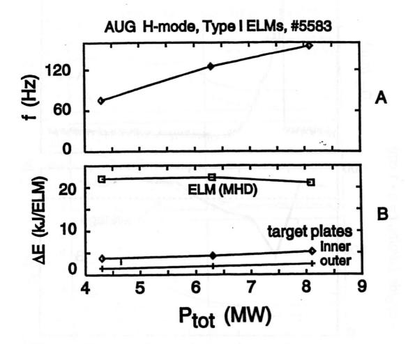
10. Energy loss due to Type I ELMs in a discharge (5583) with varying heating power: (a) the ELM frequency f (b) the energy exhausted (on average) per ELM from the plasma,  $E_{MHD}$ , and absorbed at the plates from thermography.
