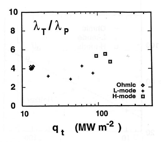
3. Ratio of upstream e-folding widths, electron temperature  $\lambda_T$  (from ECE) to parallel power density  $\lambda_P$  (from IR thermography, outer plate) in low radiation discharges as a function of parallel power density at the plate  $q_t$ .
