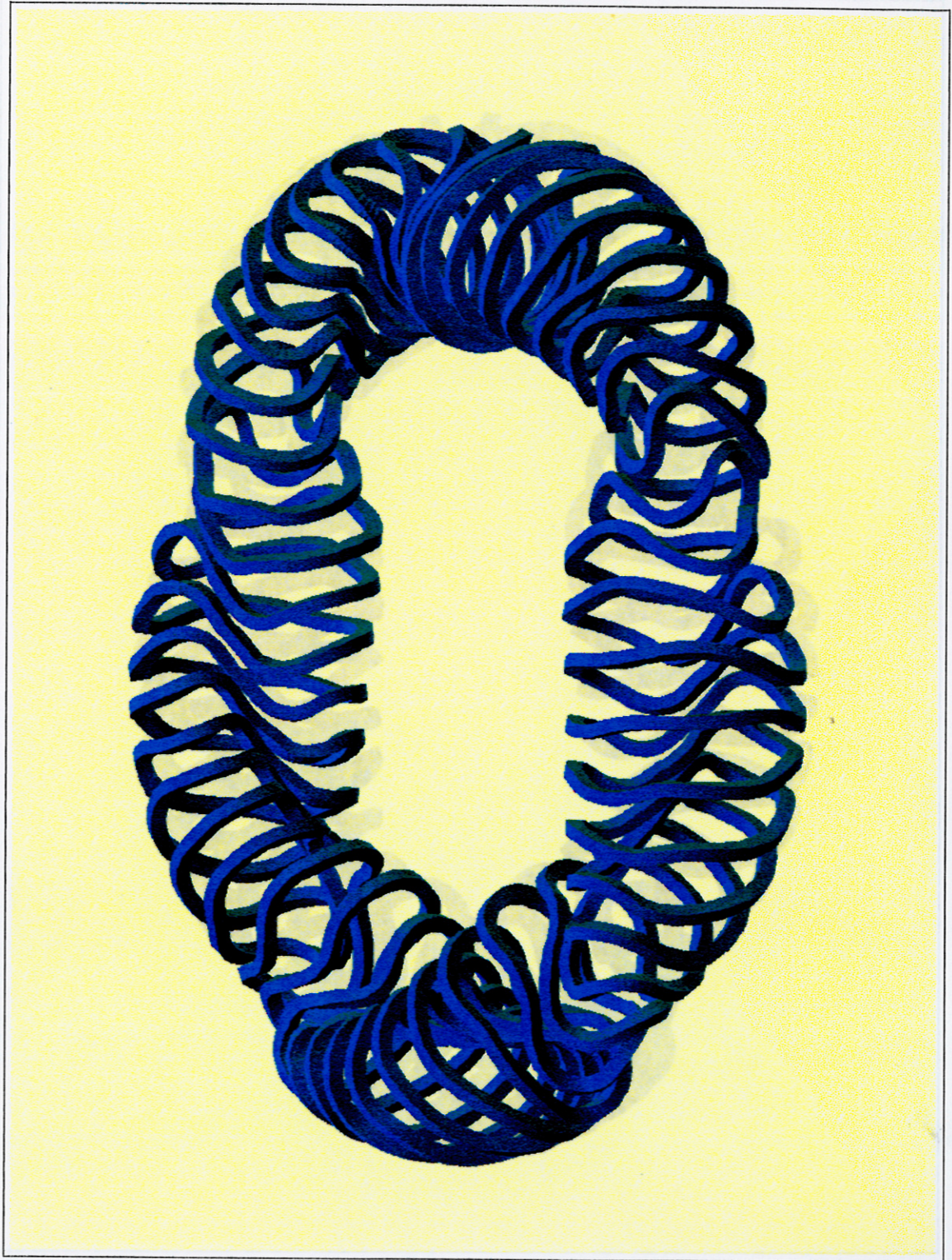
Fig. 24: Inclined view of the complete coil system, case W7-X. The figure is tilted for greatest magnification.
