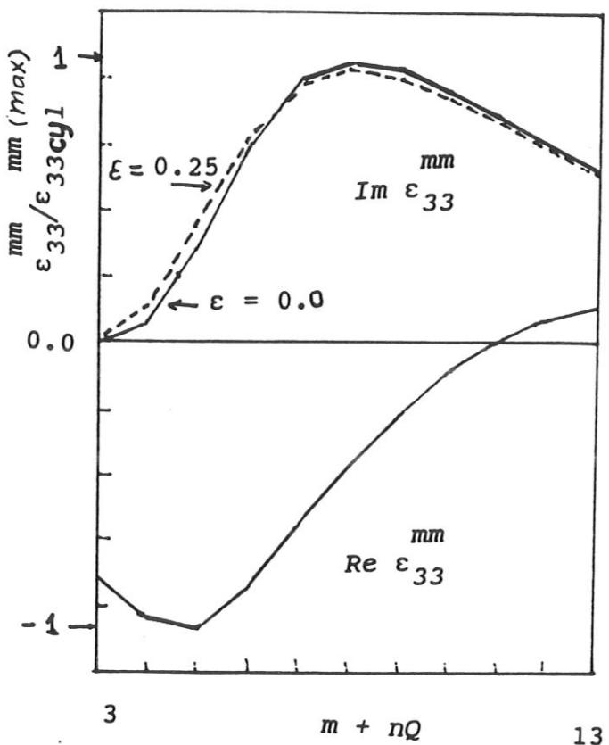
Fig.1 Dependence of parallel component of toroidal dielectric permittivity tensor normalised on cylindrical one vrs parallel component of wave vector  $k_{\parallel} RQ = m + nQ$  for  $\epsilon = 0.$  and  $0.25;$   $u_1 = 8.$
