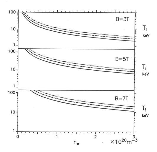
Fig. 7 Density limit for a deuterium plasma for p=70 (solid curve), p=80 (dashed curve) and p=90 (dotted curve).
