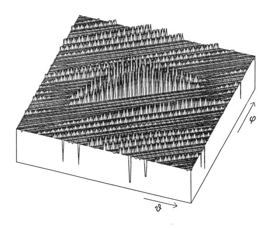
Figure 11: Alfvén ballooning solution  $U(\theta,\phi)$ . Chains of needles instead of continuous ridges are an artefact of the coarse grid. Case with very large nonaxisymmetry: F=0.7. (E=0.12128).
