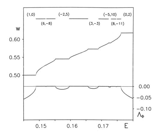
Figure 1: Upper trace: continuous spectrum of equs. (3.3), (3.6) as a function of the eigenvalue parameter  $E = \hat{\omega}^2$ . Middle trace: winding number w(E). Pairs of numbers (m,n) specify  $w = (m k_1 + n k_2)/2$  in some prominent plateaus. Lower trace: Lyapunov number  $\Lambda_{\Phi}(E)$ . (F = 0.4, G = 0.8).
