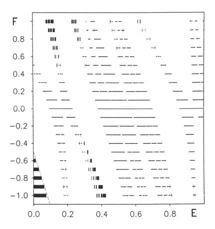
Figure 13: Overview of the spectrum of equ. (3.3) for different non-axisymmetries F. Continuous spectrum: dots. Point spectrum: bars. Dashed line:  $E_{\rm eff}=0$ . To its left:  $E_{\rm eff}<0$  in the presence of potential troughs.
