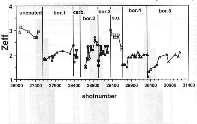
Fig. 2 Long-term dependence of Z<sub>eff</sub> on ASDEX in standard ohmic discharges with non-boronized (uncoated), boronized (bor. 1 - 5) and carbonized (carb.) walls and in start-up phases (s.u.) after venting of the vacuum vessel.
