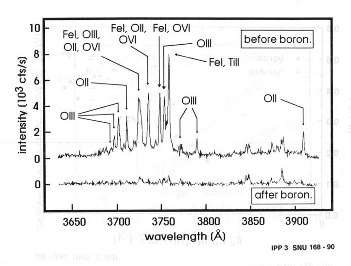
Fig. 3 Spectroscopic data measured by visible spectroscopy. After boronization the oxygen and iron line radiation disappears from the spectra.
