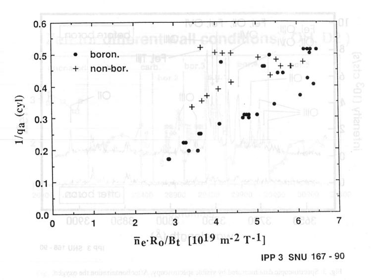
Fig. 4 The Hugill diagram  $(1/q_a \text{ versus } \overline{n_e}R/B_t, \text{ cylindrical definition for } q_a)$  shows a substantial increase in the density limit after boronization.
