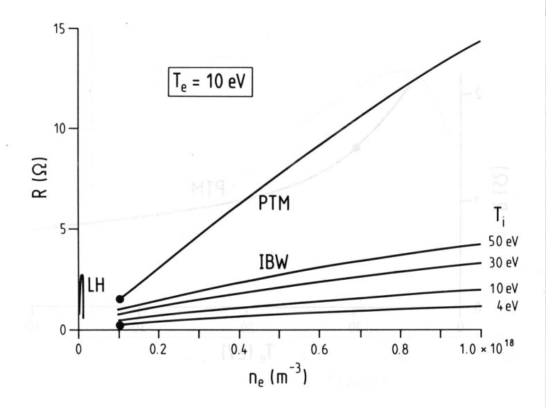
Fig.2 PTM, IBW and LH loading versus  $n_e$ . The IBW loading is shown as a function of  $T_i$ .
