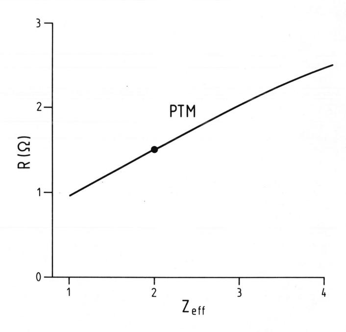
Fig.6 PTM loading versus  $Z_{eff}$ .
