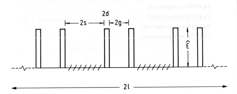
Fig.1 Idealized electric-field distribution immediately in front of the IBW antenna. Hatched regions corresponding to the Faraday-shield conductors are bordered by electric-field pulses of width 2d equal to the Debye length.
