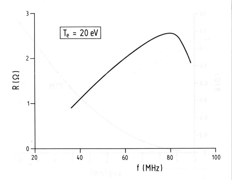
Fig.4 PTM loading versus f.
