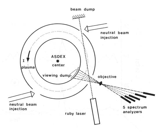
Fig. 1: Schematic set-up of the Thomson scattering system in the plasma boundary of ASDEX.
