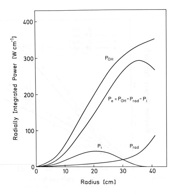
Fig.10: The radially integrated power balance for a typical ohmically heated discharge.  $\bar{n}_e = 0.28 \cdot 10^{14} \text{ cm}^{-3}$ ;  $q_a = 4.2$ ;  $B_\phi = 2.17 \text{ T}$   $P_{OH}$ : ohmic heating power  $P_i$ : power dissipated by ion heat conduction  $P_{rad}$ : radiated power as measured by bolometry  $P_e = P_{OH} - P_i - P_{rad}$ : power dissipated by electron heat conduction
