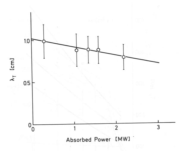
Fig. 8: The e-folding length  $\lambda_T = T_e / \frac{\partial T_e}{\partial r}$  for the electron temperature versus the absorbed beam power.
