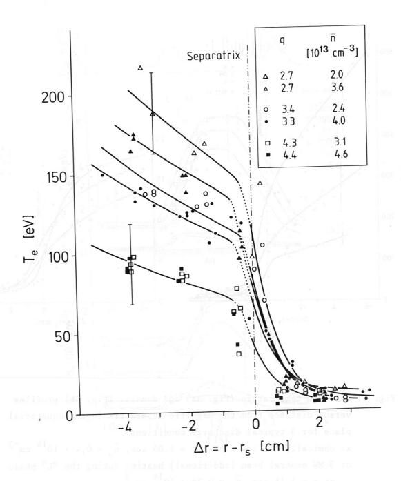
Fig. 6: Electron temperature in the plasma boundary versus distance from the magnetic separatrix for ohmically heated discharges with different q and n values. The solid lines inside the separatrix are calculated according to equ. (8). Outside the separatrix an exponential decay function was assumed.
