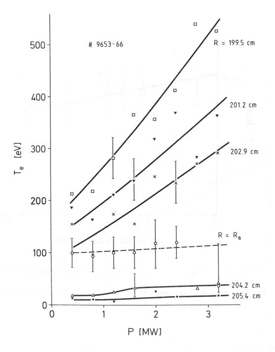
Fig. 7: Electron temperature during neutral beam heating in the "L"-phase versus the absorbed beam power (solid lines) at different radial positions, and separatrix temperature  $T_e(R=R_s)$  (dashed line). For this low q discharge (q = 2.7)  $T_e(R_s)$  is almost constant.
