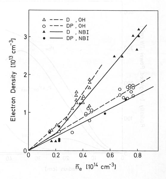
Fig. 9: Electron densities at radii  $(r_s - 1 \text{ cm}) \lesssim r \lesssim r_s$  slightly inside the separatrix versus the line averaged density  $\bar{n}_e$  for different discharge conditions.
