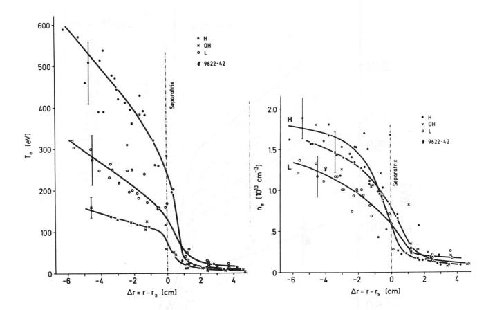
Fig. 5: Electron temperature (Fig. 5a) and density (Fig. 5b) profiles versus distance from the magnetic separatrix in the equatorial plane for 3 typical discharge conditions: x: ohmically heating alone; t = 1.05 sec,  $\bar{n}_e = 0.4 \cdot 10^{14}$  cm<sup>-3</sup> o: 3 MW neutral beam (additional) heating during the "L" phase at t = 1.15 sec,  $\bar{n}_e = 0.38 \cdot 10^{14}$  cm<sup>-3</sup>
