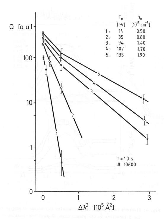
Fig. 3: Typical spectra: the photomultiplier output charge versus  $\Delta\lambda^2$  of five spectrum analysers for an ohmically heated discharge.  $\Delta\lambda$  is the spectral distance of an interference filter channel from the laser wave length.
