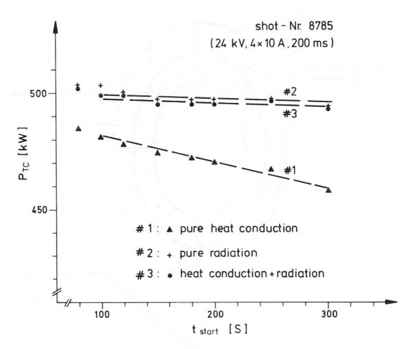
$\underline{\text{Fig. 2}}$  Calculated beam power for a shot onto the torus calorimeter for different time intervals of evaluation and different assumptions upon the cooling mechanism (see text)
