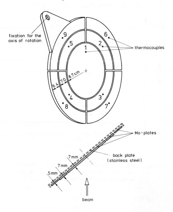
$\underline{\text{Fig. 1}}$  Layout of the torus calorimeter
