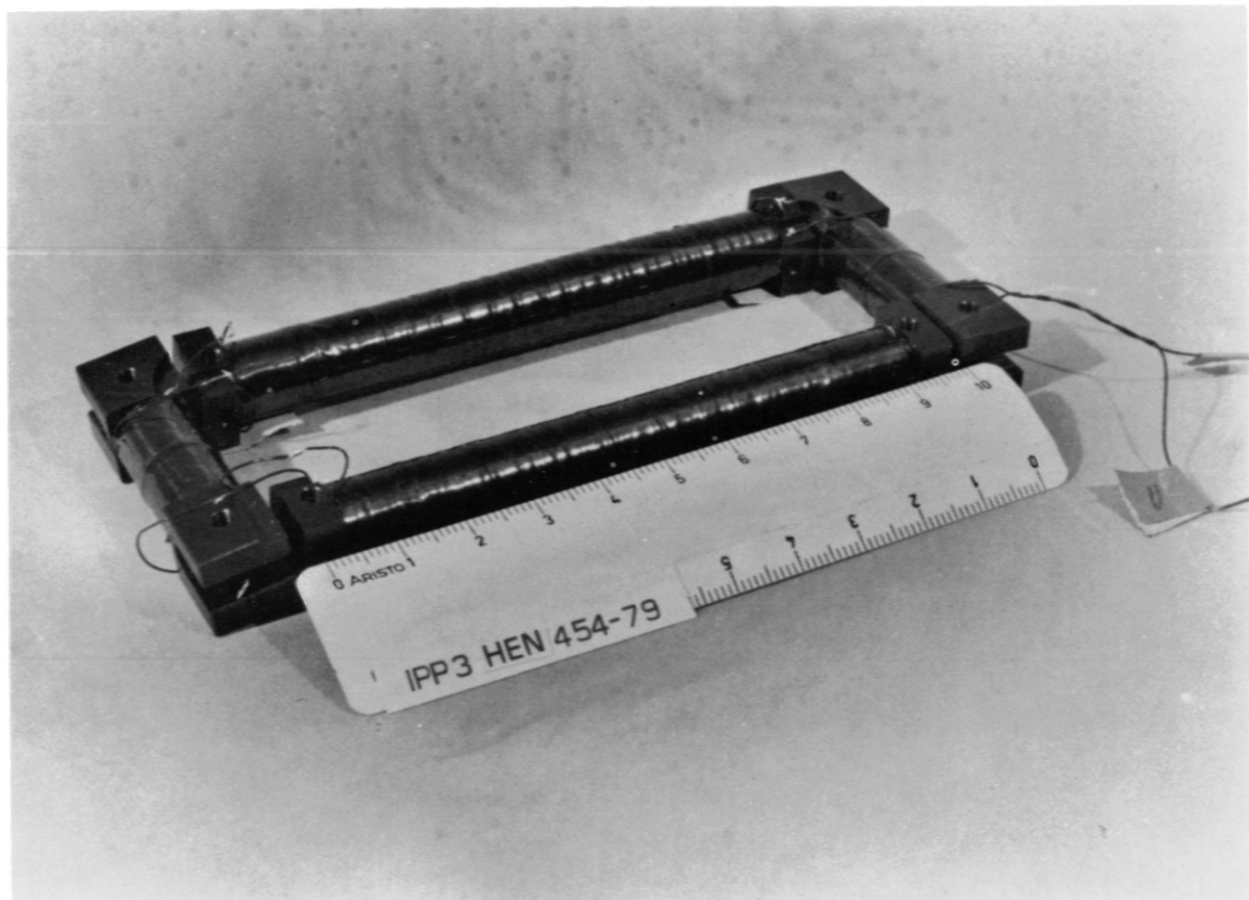
FIG.33: ROGOWSKI COIL FOR DIVERTOR COIL MOUNTED ON THE BUSBARS FOR SYMMETRICAL CURRENT MEASUREMENT (FOR CIRCUIT DESIGN SEE FIG.28)
