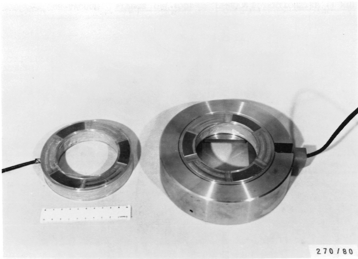
FIG: 19: PRESSURE TRANSDUCERS TO MEASURE THE WEIGHT DISTRIBUTION OF THE VACUUM VESSEL AT 8 POINTS (HIGH 20 mm)
