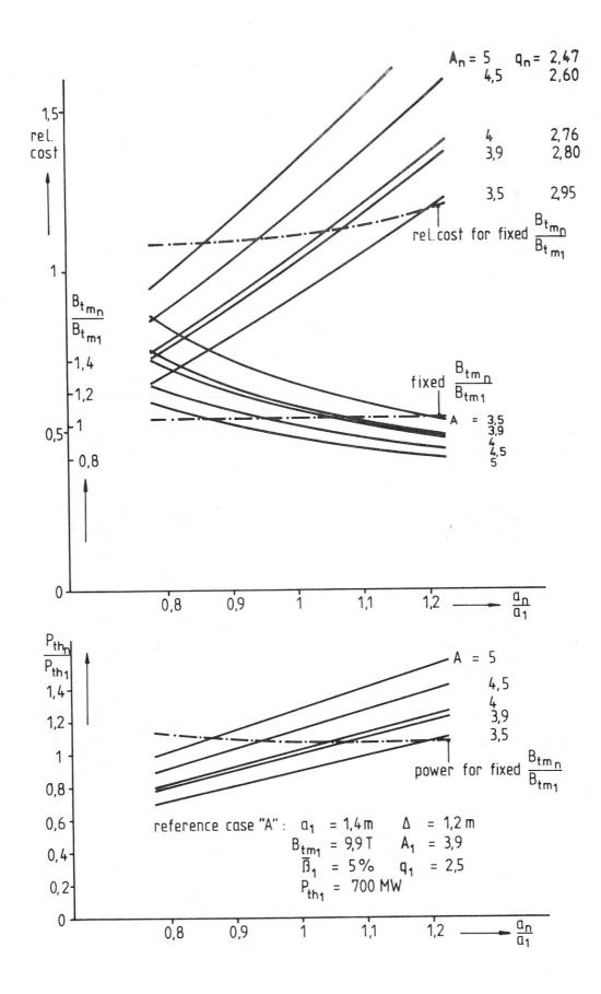
Fig. 3 INTOR cost and power scaling for X = 0.8
