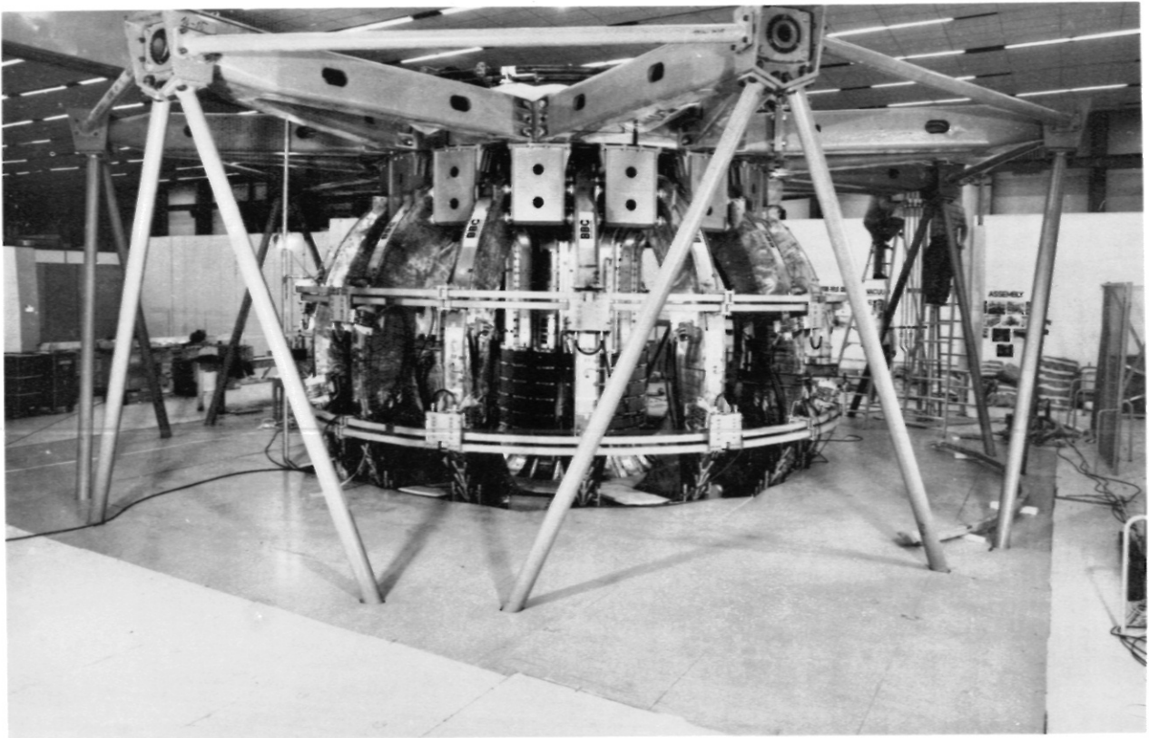
Fig.1: Toroidal field coil system, with some of the inner OH transformer coils already installed.
