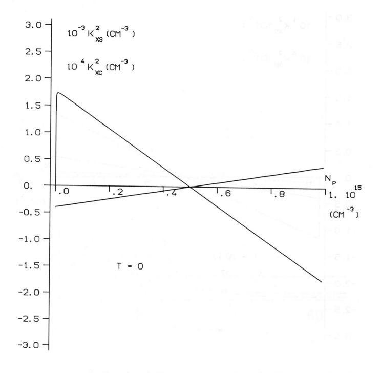
Fig. 2 The dispersion characteristics  $k_\chi^2$  versus density for both the compressional and shear waves in a cold, collisionless plasma. The value of  $n_Z$  was chosen for the Alfvén cutoff to lie midway between the plasma edge and center. The larger of the two roots corresponds to the shear wave.
