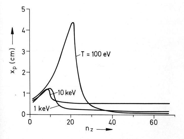
Fig. 4 Attenuation distance for which the shear wave amplitude drops to one-tenth of its value at the plasma surface versus  $n_z$ . The humps to the left occur because at the low  $n_z$  values  $e^{-}$  becomes less than unity and the wave becomes propagating from the plasma edge till the Alfvén cutoff layer.
