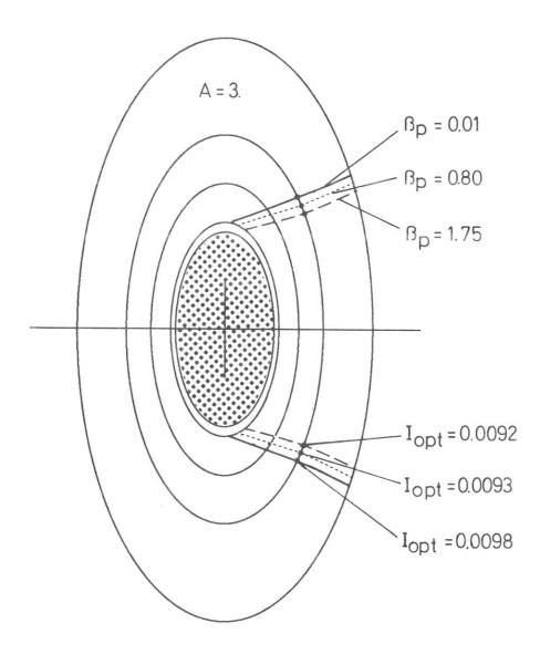
Fig. 6: Optimum loop positions and feedback currents  $\label{eq:currents} \text{for several } \textbf{B}_{p} \quad .$
