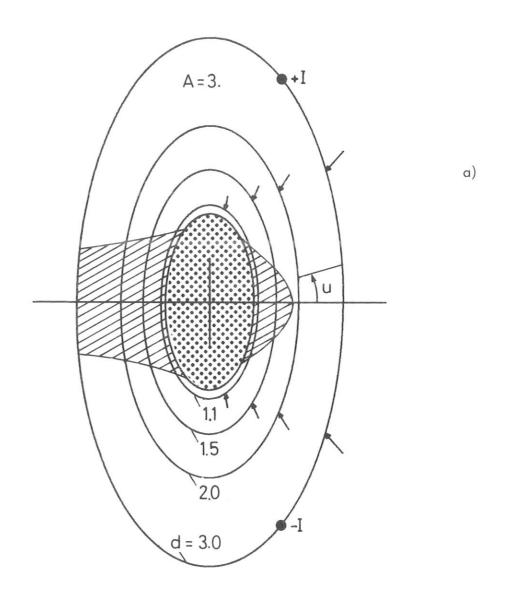
Fig. 2: Effective (blank) and ineffective (hatched) loop positions for A = 3.
