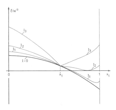
Fig. 9: Energy  $\delta W^a$  versus mode amplitude  $\mathbf{x}_1$  for several values of feedback current J.
