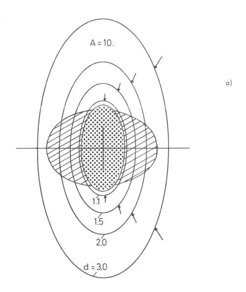
Fig. 3: Effective and ineffective loop positions for A = 10.
