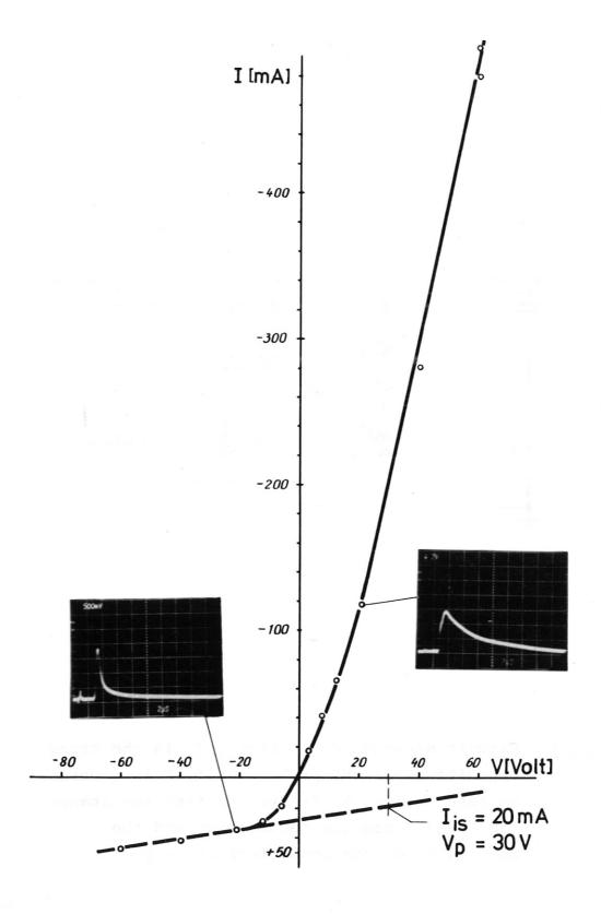
Fig. 2 Typical oscillograms and current-voltage characteristic obtained from a 1 mm dia-disc probe. Target: stainless steel plate; laser energy: 2 J, normal incidence.
