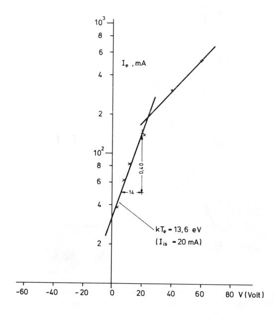
Fig. 4 Plot of log  $I_e$  vs. V.  $I_{is} = 20$  mA ist used to obtain  $I_e = I - I_{is}$  from Fig. 2.
