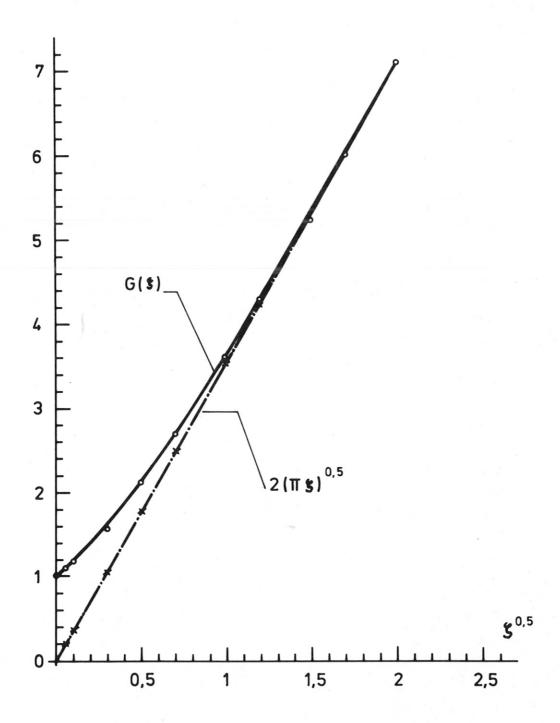
Fig. 5 Variation of the function  $G(\xi)$  with respect to the parameter  $\xi^{1/2} = (\frac{m}{2kT})^{1/2}$ .
