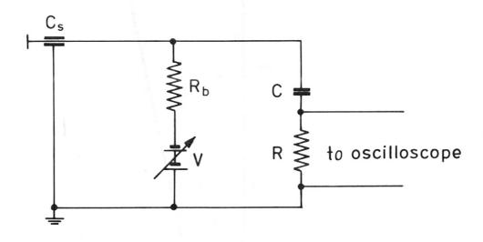
Fig. 1 Circuit diagram of the probe. C<sub>s</sub> is the stray capacitance of the probe itself, V is a variable voltage source, R<sub>b</sub> is the charging resistance, and C and R are the capacitance and the resistance of the load, respectively.
