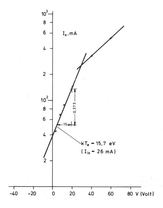
Fig. 3 Plot of log  $I_e$  vs. V.  $I_{is} = 25$  mA is used to obtain  $I_e = I - I_{is}$  from Fig. 2.
