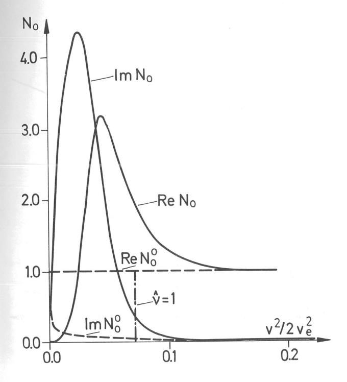
Fig 1. Resonance function  $N_o$  (  $\hat{\omega}$ ,  $\hat{v}$  ) vs.  $v^2/2v_e^2$ ;  $\hat{v} = (1/k_\lambda) (v_e/v)^4$ ,  $\hat{\omega} = \omega/kv$ ;  $\omega/kv_e = 0.03$ ,  $1/k_\lambda = 0.02$ . Collisionless theory  $N_o^o$  and its cutoff in earlier theories.
