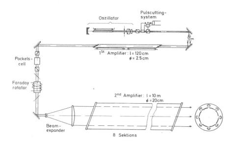
Fig. 2 Schematic set-up of Asterix III
