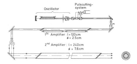
Fig. 1 Schematic set-up of Asterix II
