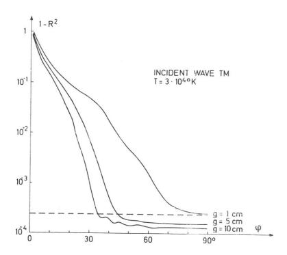
Fig. 2 Transmitted energy as a function of and T for an incident TE wave.
