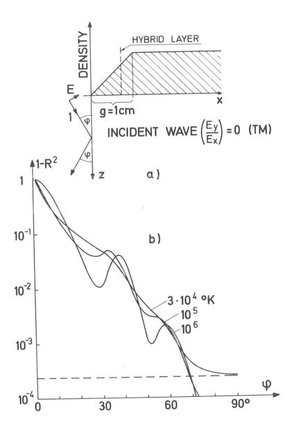
Fig. 1 Transmitted energy (1-R<sup>2</sup>) as a function of the angle of the incident TM wave with the vacuum-plasma interface for several values of temperature T.
