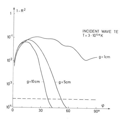
Fig. 4 Transmitted energy as a function of and "g" for an incident TE wave.
