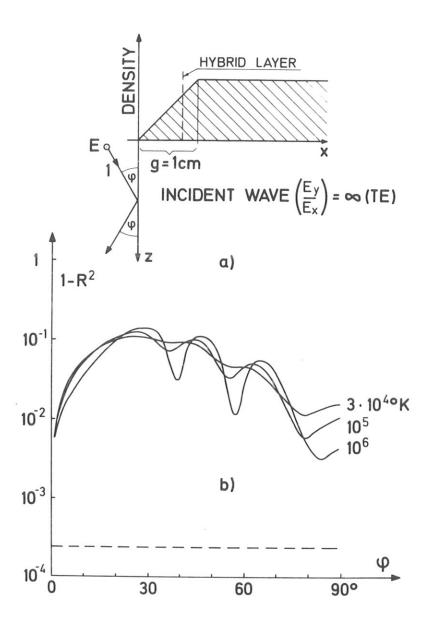
Fig. 3 Transmitted energy as a function of and the profile width "g" for an incident TM wave.
