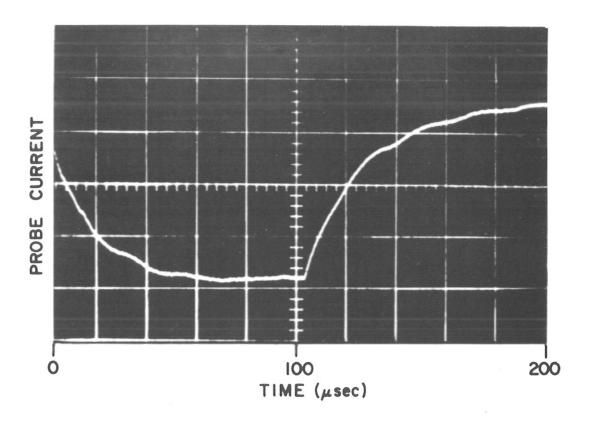
Fig. 6 Plasma heating and cooling characteristic interval on application and removal of the applied field
