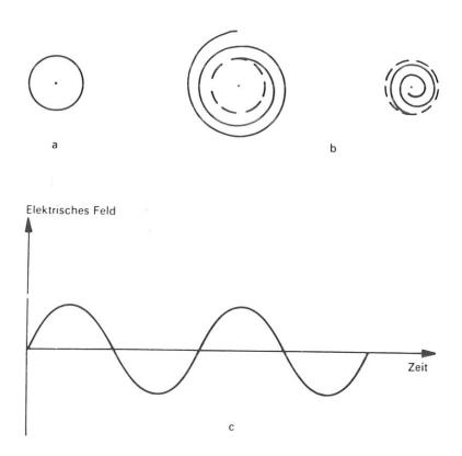
Fig. 2 . Spiraling motion due to cyclotron frequency electric field
