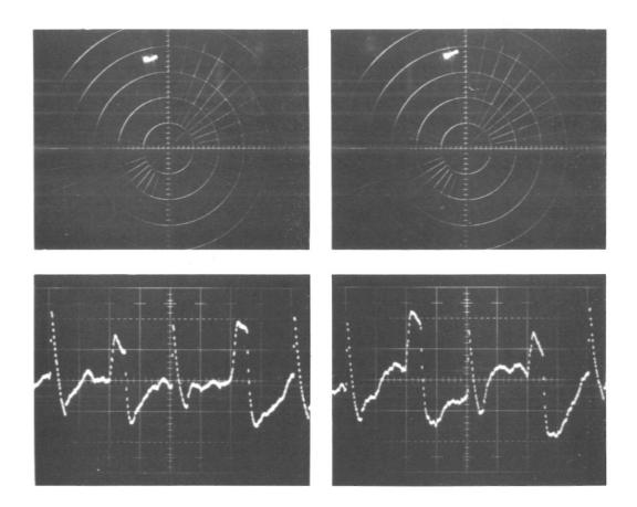
Fig. 13 Typical diamagnetic (flat topped) and calibration signals.
