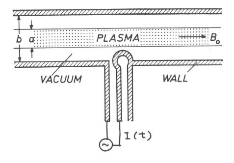
Fig. 14 A plasma filled waveguide driven by a current source.
