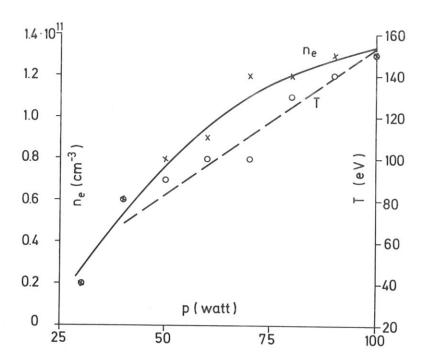
Fig. 12 Plasma density and electron temperature as a function of input noise power.
