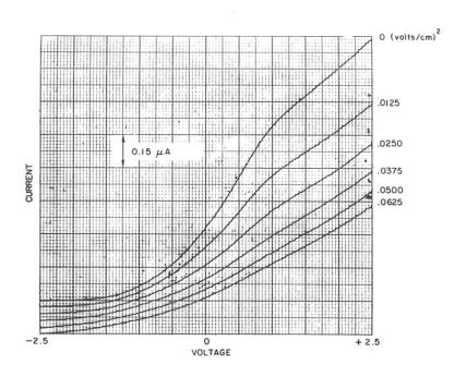
Fig. 7 Langmuir probe curves obtained on an x-y recorder
