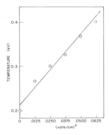
Fig. 8 Applied field strength vs plasma temperature
