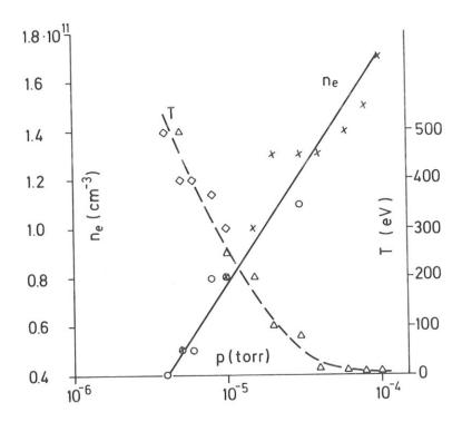
Fig. 11 Plasma density and electron temperature as a function of pressure.
