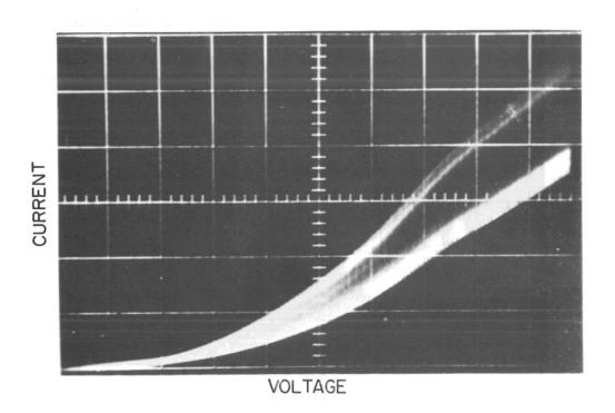
Fig. 5 Langmuir probe curves obtained on an oscilloscope
