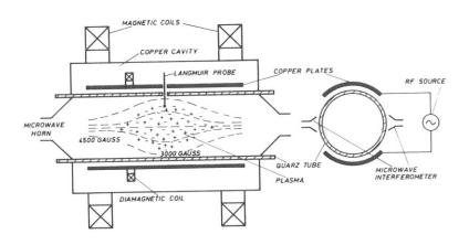
Fig. 9 Schematic of the experimental arrangement
