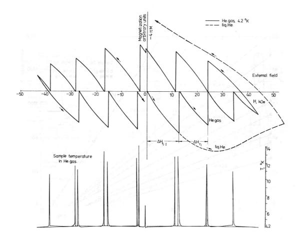
Fig. 3 XY<sub>1</sub>Y<sub>2</sub> recording of magnetization and temperature vs field of a stack of Nb<sub>3</sub>Sn tape discs in liquid helium and helium gas at 4.2°K
