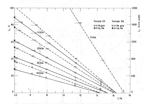
Fig. 2 Critical current vs temperature with different magnetic fields as a parameter for diffusion processed Nb<sub>3</sub>Sn tape
