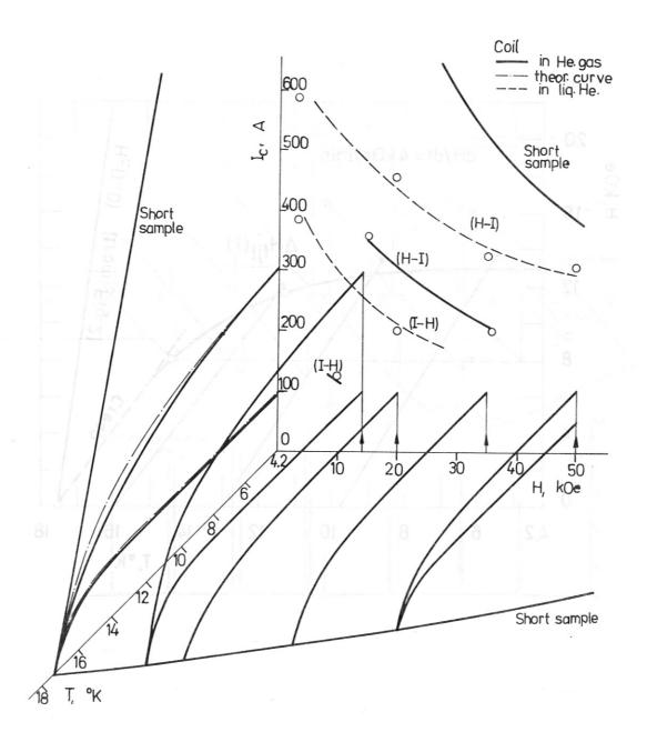
Fig. 5 Three-dimensional (HIT) representation of a number of tests on a Nb<sub>3</sub>Sn small sample coil in helium gas and in liquid helium.
