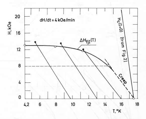
Fig. 4 First flux jump interval ( $\Delta H_{fjI}$ ) as a function of temperature in helium gas for a stack of Nb<sub>3</sub>Sn tape discs (as in Fig. 3)
