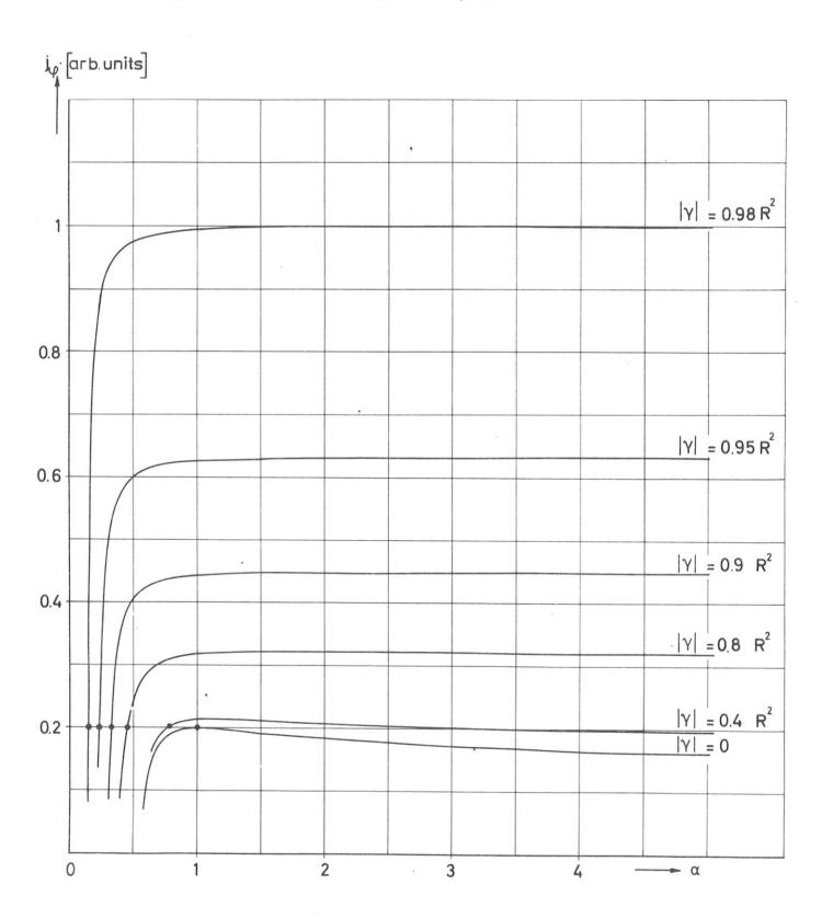
Fig. 2 The limit of the toroidal plasma  $\beta$  versus  $\alpha$  for different values of IyI. IyI is proportional to the poloidal current density;  $\alpha$  denotes for a given IyI a certain eccentricity of the elliptic near axis cross sections of the magnetic surfaces. The values of  $\alpha$  corresponding to a circular cross section are marked with a point.
