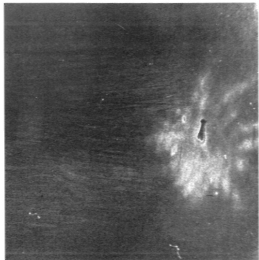
Figs. 19 - 22 Beam structure at outlet of brass cone with its axis inclined at an angle \alpha to the beam direction
