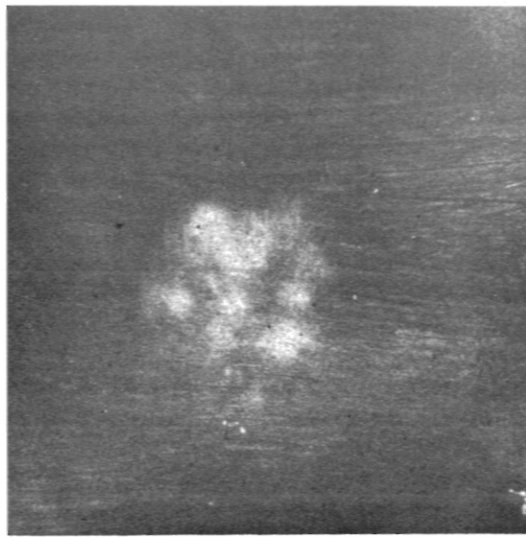
Fig.18 Beam structure at outlet of cone made of silver paper
