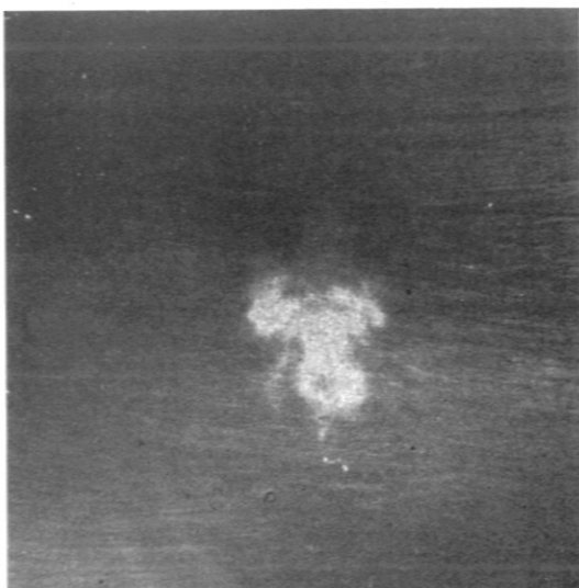
Figs. 19 - 22 Beam structure at outlet of brass cone with its axis inclined at an angle \alpha to the beam direction
