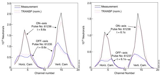
**Figures 3 and 4.** Neutron camera profiles for low power (left) and high power (right) high  $q_{95}$  regime showing on-axis (peaked) and off-axis (flattened) T deposition and comparing simulation with measurement (Bicron).
