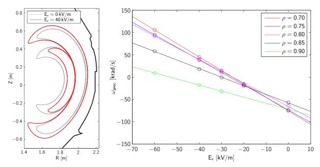
Figure 1: Effect of a constantFigure 2: Effect of a constant radial electric field on the precessionradial electric field on orbitdrift frequency (positive sign indicates co-injection direction) for dif-widths.ferent birth radii.
