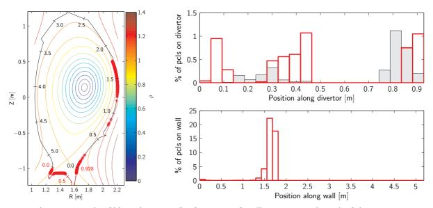
Figure 3: Fast particle (60keV) losses to the divertor and wall structures. The poloidal cross section on the left illustrates the wall and divertor coordinates used in the histogram on the right and in figures 4 and 5. The red asterisks show the hit points in the presence of ripple. In the histogram, red and grey bars show the results with and without ripple, respectively. The percentages don't add up to 100% because the thermalized particles don't show up in the histogram.
