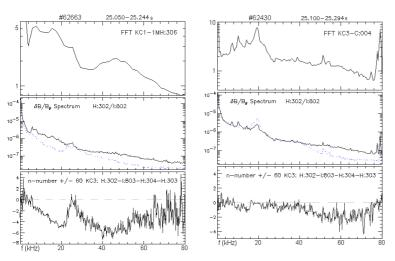
Fig.7 Magnetic power spectra, out/in coil signals, estimated toroidal mode numbers for ELM-free phases in identity plasmas to C-Mod (left) and ASDEX-U (right).
