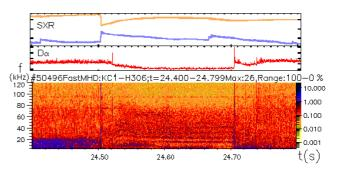
Fig.2 SXR, divertor Dα, power spectrum of magnetic fluctuations spanning an ELM-free H-mode interval in a very similar ICRH plasma. "Washboard" modes are visible as multiple coherent frequency stripes.
