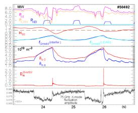
Fig.1 Input power, normalized confinement and density, central and edge density, divertor  $D\alpha$ , reflectometer fluctuation amplitude, for two ICRH ELM-free H-mode phases.
