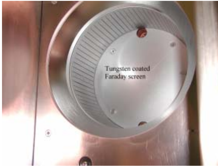
Fig. 3.3. Tungsten coated faraday screen is sitting inside the driver, attached with the expansion region.
