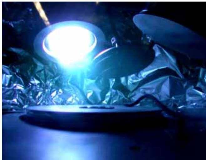
Figure 2.4. Deposition plasma in sputter device
