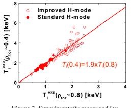
Figure 2. Experimentally measured ion temperature at  $\rho_{tor}=0.4$  versus those at  $\rho_{tor}=0.8$  for standard and improved H-mode discharges.
