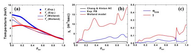
Figure 3. Pulse 58323 at JET; experimental and calculated ion and electron temperature profiles (a), corresponding ion heat conductivity (b),  $E \times B$  shearing rate and linear growth rate (c) at premature and fully developed improved H-mode regime.
