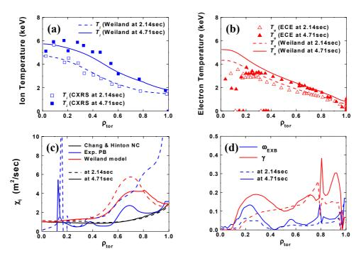
Figure 1. Pulse 17870 at ASDEX Upgrade; experimental and calculated ion (a) and electron (b) temperature profiles, corresponding ion heat conductivity (c),  $E \times B$  shearing rate and linear growth rate (d) at premature and fully developed improved H-mode regime. For  $\rho_{tor} > 0.8$ , the transport calculation is not performed.
