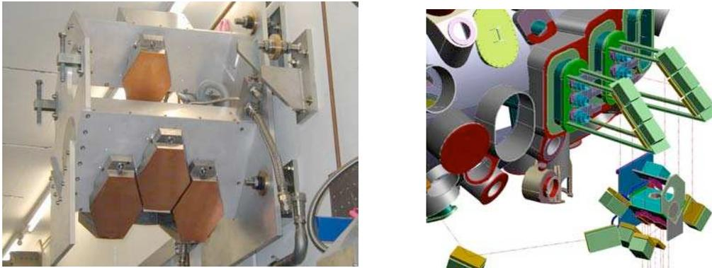
**Fig. 3:** Beam combining optics unit (left) and design of the beam distribution and feeding system for the front-steering launcher (right)
