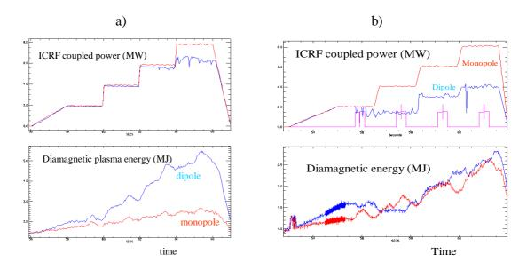
**Fig.1** Evolution of coupled power and plasma energy for a) SFE 2.8 MA (#52672, #52670) and b) DOC-U 2 MA (#58944, #58949) configurations in a power ramp-up to 8 MW with steps of 2 MW.
