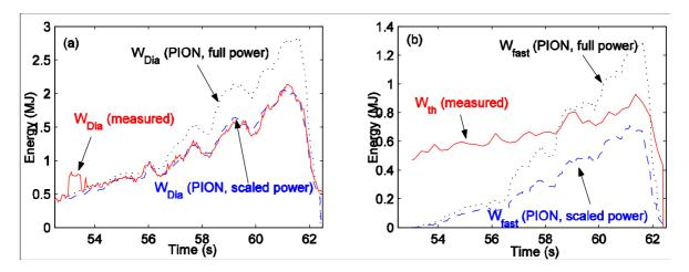
**Fig.2** (a) Diamagnetic energy content from measurements (—) and from PION calculations with full power (…) and with optimally scaled power (---) to match the measured  $W_{dia}$ . (b) Thermal energy content (—), fast ion energy content calculated by PION using full injected power (…) and optimally scaled power (---).
