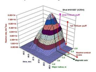
Fig.6. 14 MeV neutron profile with ICRH Tritium fundamental heating showing that the neutron emission centre is shifted toward the high field side with respect to the magnetic axis.
