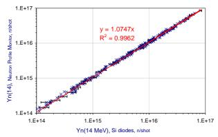
Fig.5 Comparison of 14 MeV neutron yield measured by Neutron Profile Monitor (Bicron detectors) and Si diodes (~450 TTE shots)
