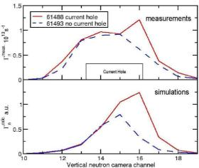
Fig.7. Comparison of calculated and measured profiles for the vertical 14 MeV neutron camera for on-axis tritium beams. DT neutron profiles during on-axis tritium beam blip indicate an outward displacement of neutron emission (measured on the top, calculated on the bottom).
