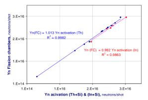
Fig. 2. Calibration factors for four different Silicon diodes (DT neutron monitors) derived from activation measurements.
