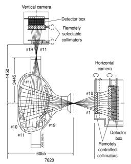
Fig. 4. Schematic view of JET neutron profile monitor
