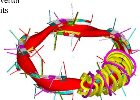
one magnetic field period: 10 modular coils, 4 ancillary coils
