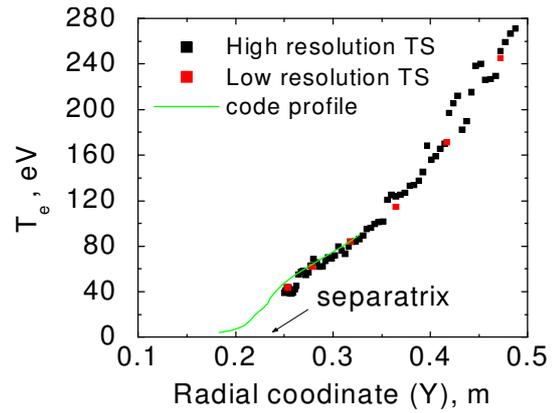
Fig.3 (b). Comparison of calculated electron temperature profile and TS data at the inner midplane for shot 5498.
