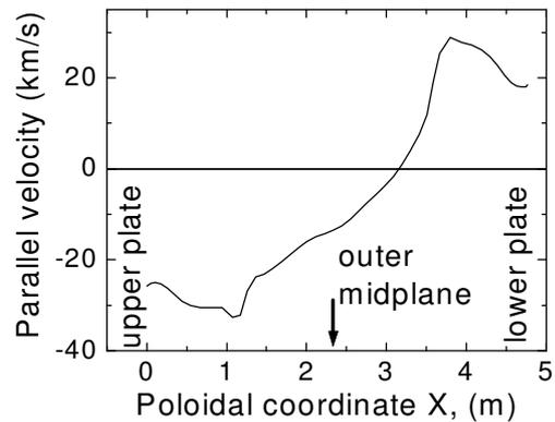
Fig.7. Poloidal profile of parallel velocity in the outer SOL for shot 7138.
