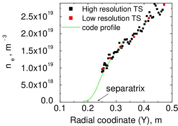
Fig.3 (a). Comparison of calculated density profile and TS data at the inner midplane for shot 5498.
