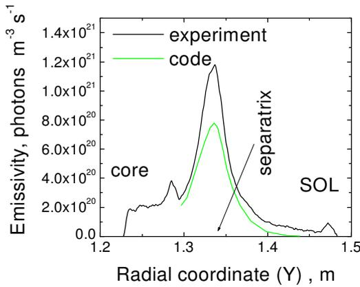
Fig.4. Radial profile of  $D_{\alpha}$  emission at the outer midplane. Code calculation for shot 5498.
