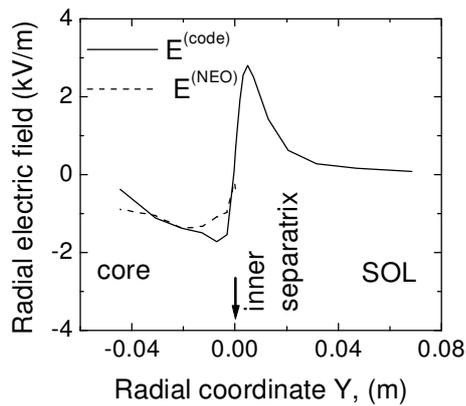
Fig.6. Radial electric field profile for shot 5498.
