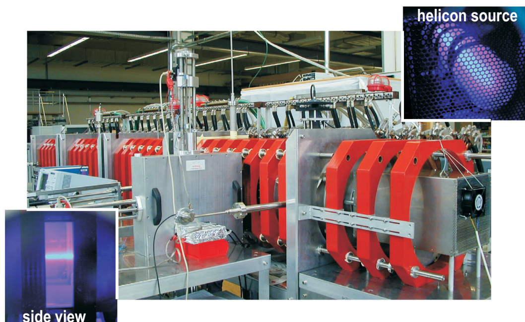
Figure 4.1: Picture of the linear magnetised plasma experiment VINETA in configuration for rf plasma production. The insets show the helicon discharge mode in argon seen through an optical bandpass filter around (442 \pm 5) nm.
