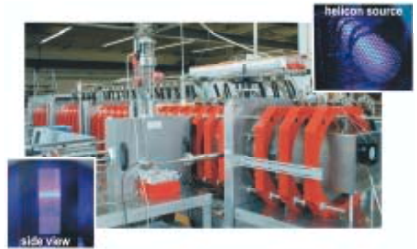
Figure1: Full view of the VINETA device. The magnetic field coils (red) can be adjusted along the axis. The helicon plasma source is installed on the right-hand side.
