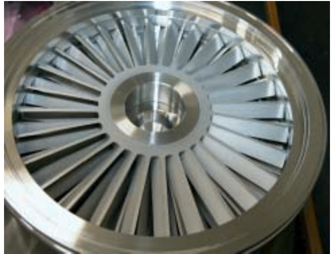
Figure 17: Robust rotor of the new TMPs
