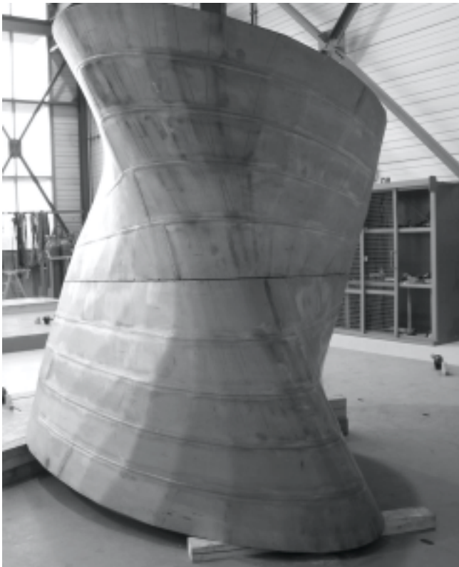
Figure 3: Half-module of the plasma vessel (by courtesy of Deggendorfer Werft und Eisenbau GmbH)
