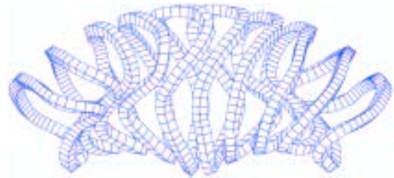
Figure 2: View from top of one period of the coil set (winding packs) of HSR 3/15.
