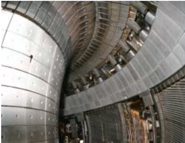
Figure 16: Tungsten coated inner heat shield and upper PSL
