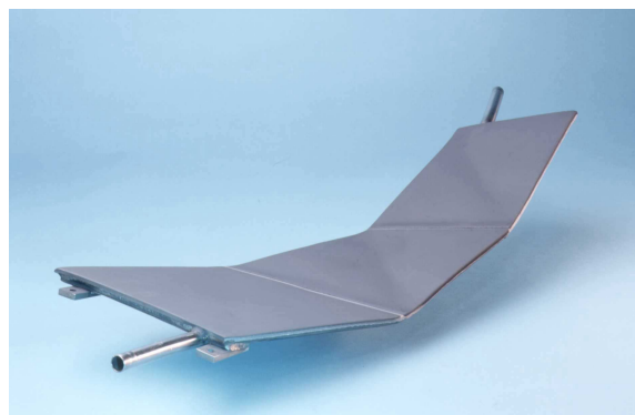
Figure 4: Prototype of \text{B}_4\text{C} covered first wall panel (manufacturer: Plansee/Deggendorfer Werft)
