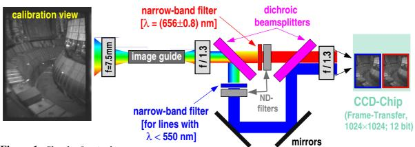
Figure 1: Sketch of optical setup
