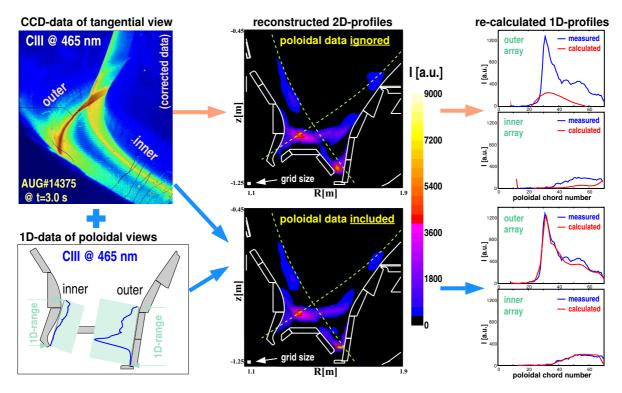
Figure 2: 2D-reconstruction with and without including profile information from poloidal views
